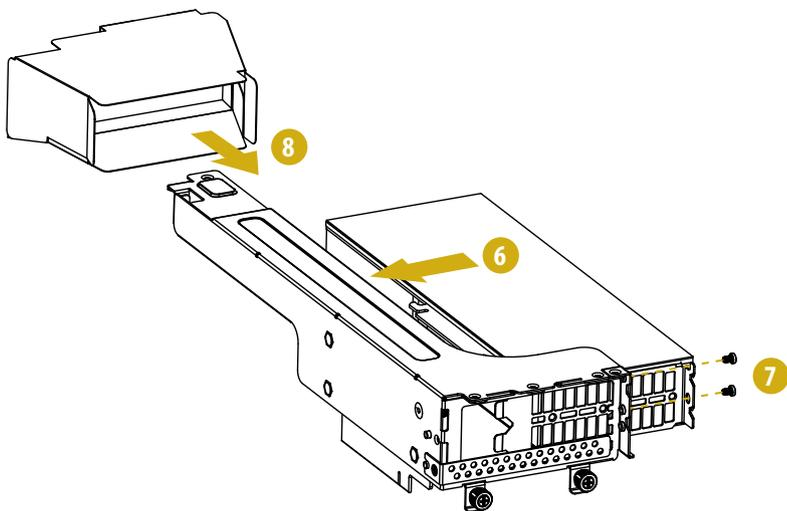
9. Install the riser card assembly to the chassis. Align the plate of the card with the openings in the back of the chassis.
