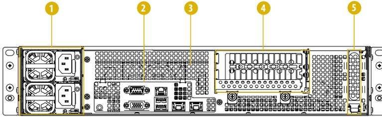
Redundant PSU 1+1: Only one PSU is allowed to be removed while the server is running.
