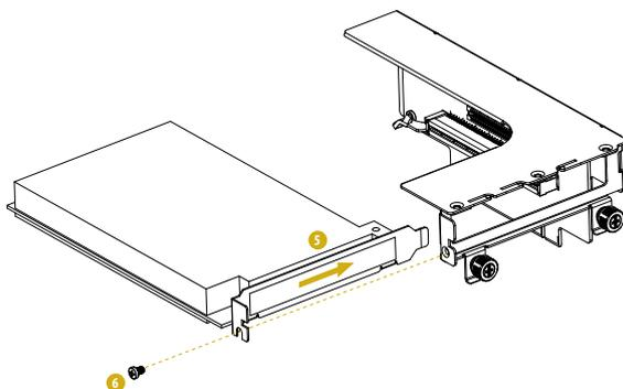
7. Install the LAN card assembly to the chassis. Align the plate of the LAN card with the openings in the back of the chassis.
