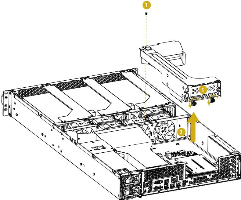
3. Remove the screws securing the slot cover to the assembly.
