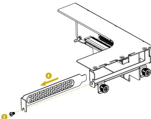
5. Install the LAN card into to the riser-card assembly.
