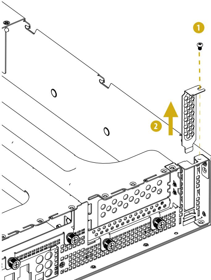
3. Install a PCIE card into to the slot.
