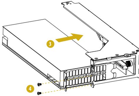
5. Install the riser card assembly to the chassis. Align the plate of the add-on card with the openings in the back of the chassis.
