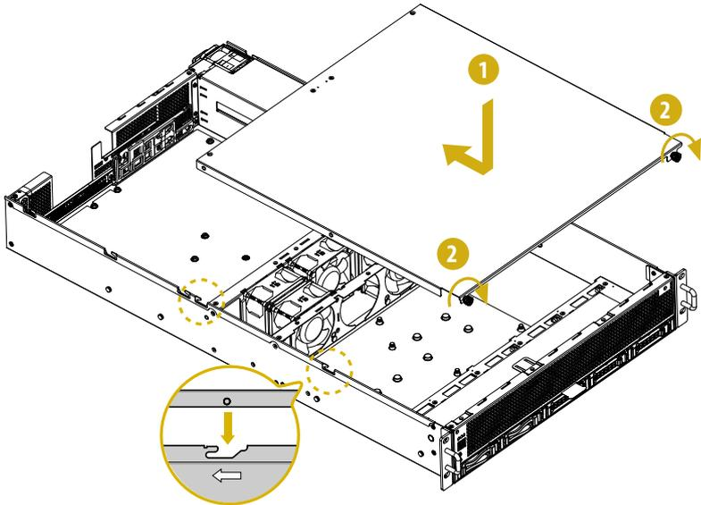
3. Then lower the top rear cover on the chassis, making sure the side latches align with the cutouts. Slide the top front cover toward the FRONT of the chassis.
