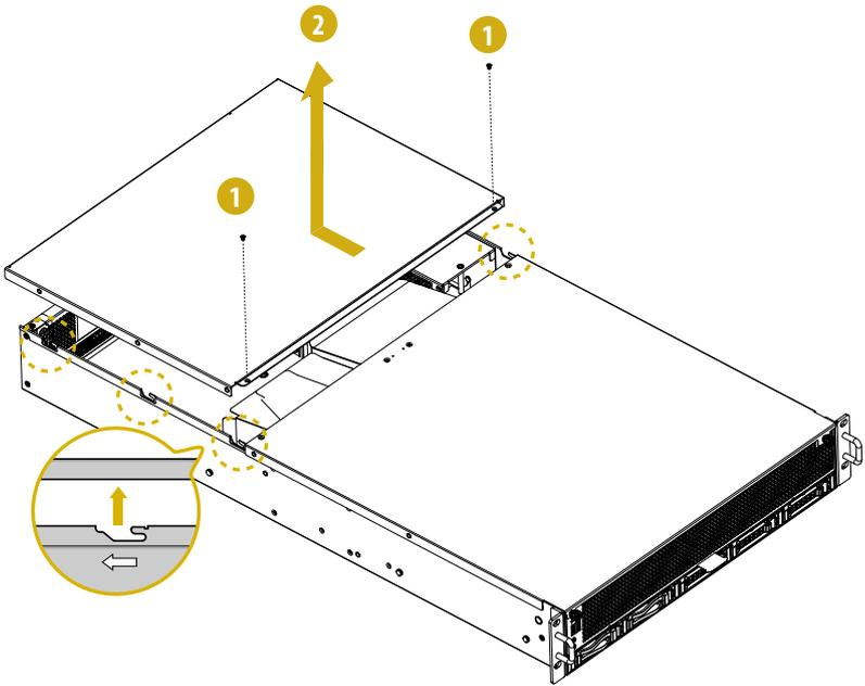
3. Release the thumbscrews that secure the top front cover to the chassis.
