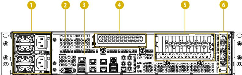
Redundant PSU 1+1: Only one PSU is allowed to be removed while the server is running.
